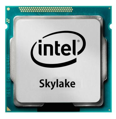
Intel's Turbo Boost 2.0 Technology, and it's equipped with 8MB of Intel Smart Cache memory.
