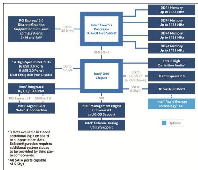
Gamers also stand to benefit from an abundance of PCIe lanes available to Haswell-E processors. The 5960X and 5930K both have 40 lanes at their disposal, putting a 4-way SLI or CrossFire setup within easy reach. The 5820K is limited to 28 lanes, but that's more than enough for a powerful multi-GPU setup.
